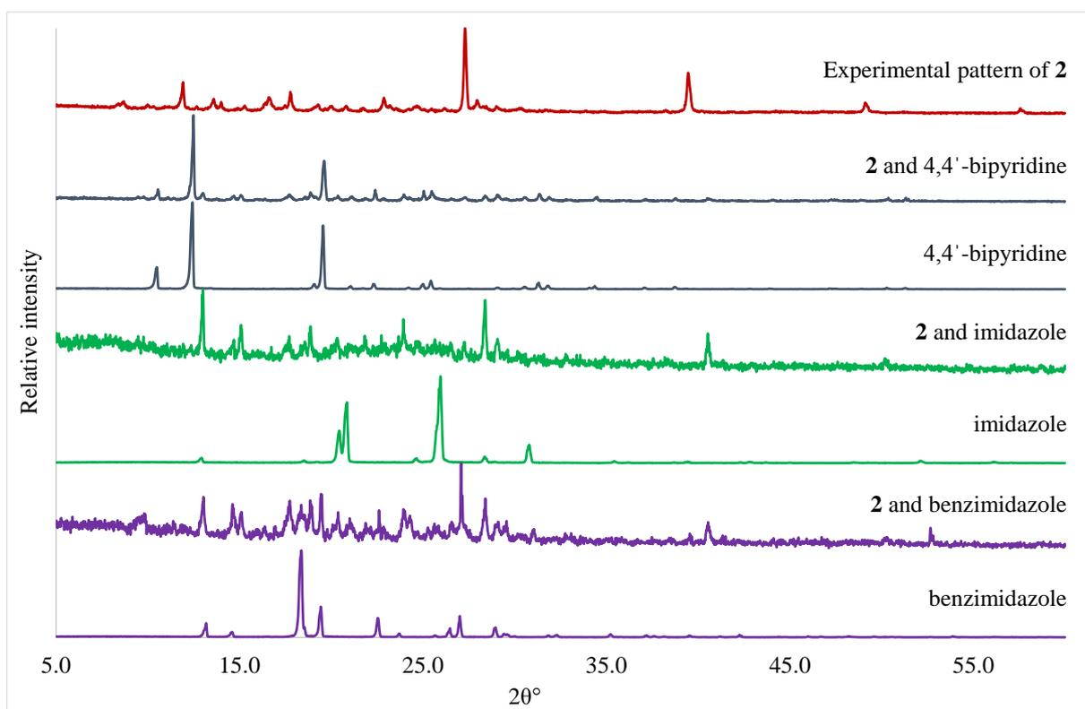
**Figure S1** PXRD results of the grinding experiments with **2**. The powder patterns of the products either correspond to that of **2** or the co-crystal former.
