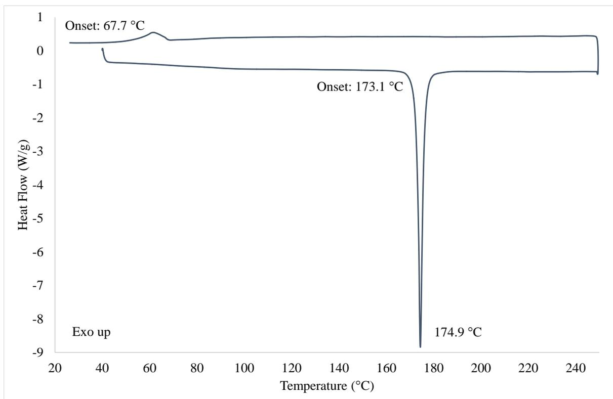
**Figure S12** DSC analysis of the product of **11** and **12**. The melting point of **11/12** is lower than that of both the reagents.
