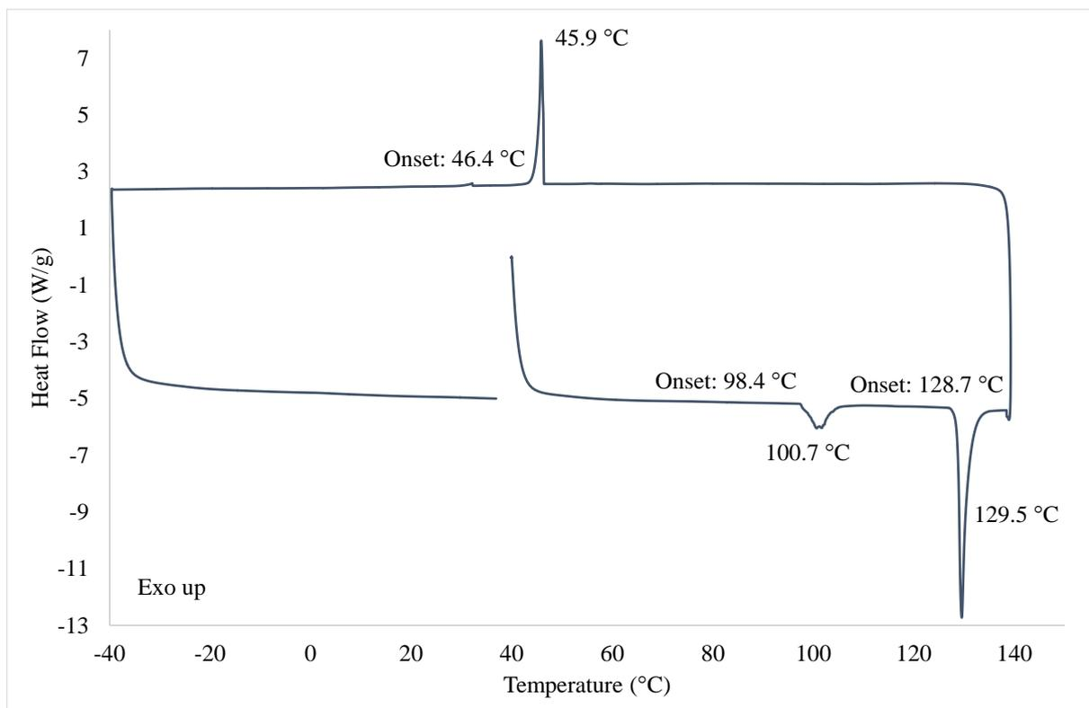
**Figure S7** DSC analysis of the triclinic form of hexakis(4-fluorophenoxy)cyclotriphosphazene (**9**). The triclinic form (**9** $\beta$ ) converts to **9** $\gamma$  around 100 °C before the melt at 129.5 °C.
