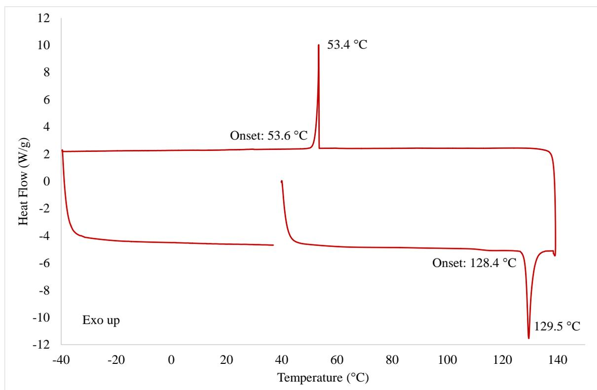
**Figure S6** DSC analysis of the monoclinic form of hexakis(4-fluorophenoxy)cyclotriphosphazene (**9**), with a melt at 128.4 °C and a recrystallization event upon cooling at 53.6 °C. This structure undergoes single-crystal to single-crystal polymorphic transitions where **9 $\alpha$**  (the monoclinic *P* form) converts to **9 $\gamma$**  between 115 and 125 °C before melting.
