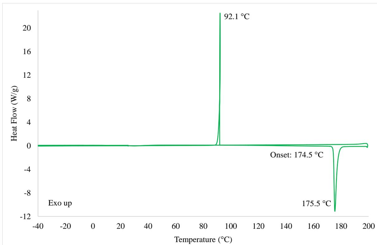
**Figure S9** DSC analysis of hexakis(4-bromophenyl)cyclotriphosphazene (**11**), with a melt occurring at 174.5 °C and a recrystallization event upon cooling at 92.1 °C.
