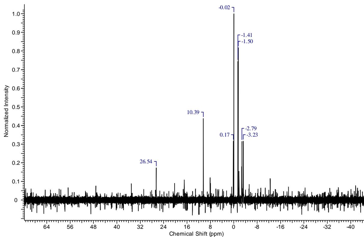
**Figure S5** The  $^{31}\text{P}$  NMR spectrum of the precipitate formed when the product of mechanochemical synthesis between **2** and benzimidazole is dissolved in THF. Multiple peaks for phosphorous indicates that ring cleavage could have occurred.
