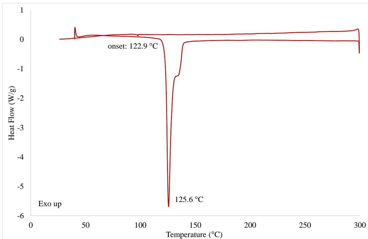
**Figure S11** DSC analysis of the melt product (**9/10**) of the fluoro and chloro derivatives. Melting occurs before the melting point of the fluorophenoxy derivative (129 °C).
