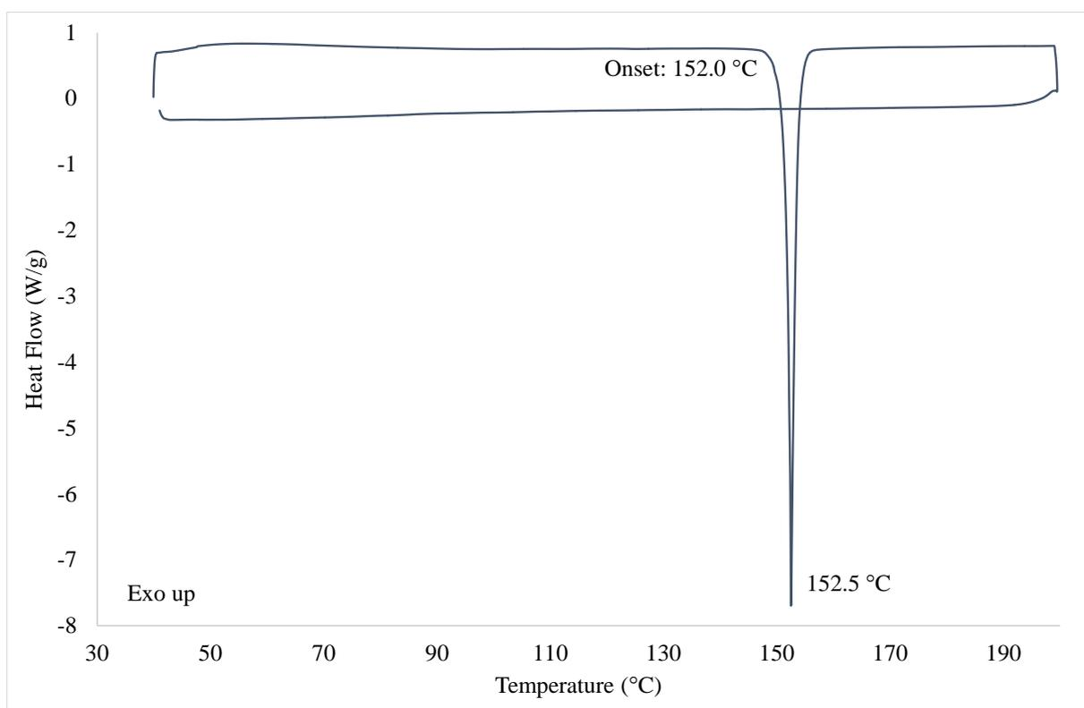
**Figure S8** DSC analysis of hexakis(4-chlorophenyl)cyclotriphosphazene (**10**), with a melt occurring at 152.0 °C.
