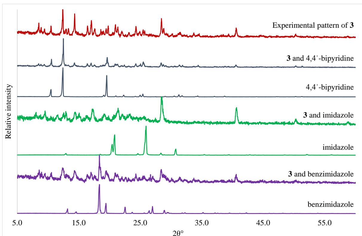
**Figure S2** The PXRD results of the mechanochemical experiments between **3** and 4,4'-bipyridine, imidazole and benzimidazole. In most cases there appears to be an agreement between the patterns of the product and 4,4'-bipyridine, imidazole and benzimidazole.
