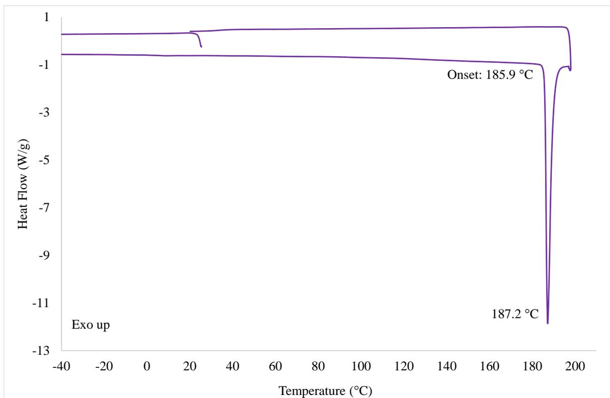
**Figure S10** DSC analysis of hexakis(4-iodophenyl)cyclotriphosphazene (**12**), with a melt at 185.9 °C.
