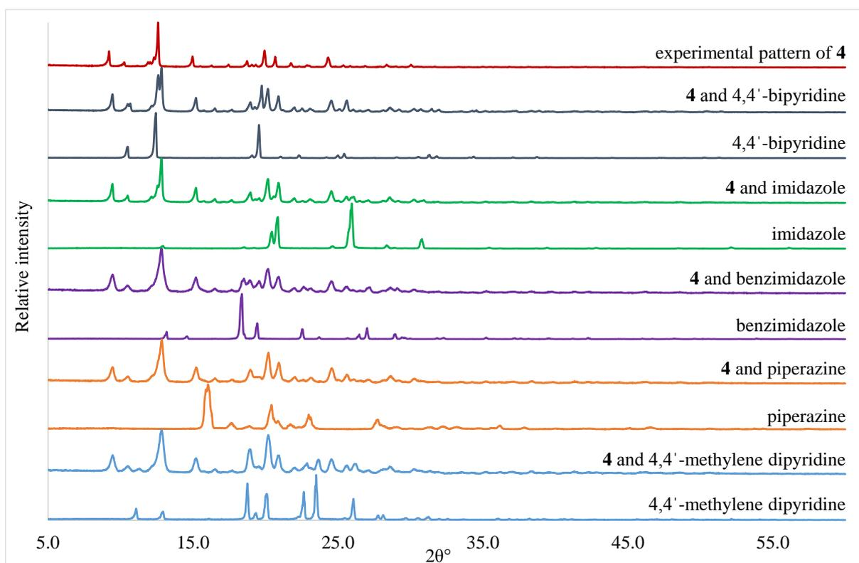
**Figure S3** The PXRD results of mechanochemical experiments with **4**. In all cases the product of the grinding experiment corresponds to the powder pattern of **4**, indicating that no co-crystals were formed.
