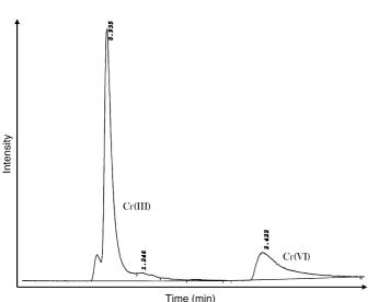
Figure 2 Typical chromatogram achieved with AG 9 and AS 9 columns (sample: 20 mg  $L^{-1}$  Cr(III) and 20 mg  $L^{-1}$  Cr(VI)).
