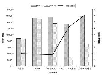
**Figure 1** Comparison of the sensitivity and resolution obtained by various anion chromatographic systems (sample:  $20 \text{ mg } \text{L}^{-1} \text{ Cr}(\text{III})$  and  $20 \text{ mg } \text{L}^{-1} \text{ Cr}(\text{VI})$ ).
