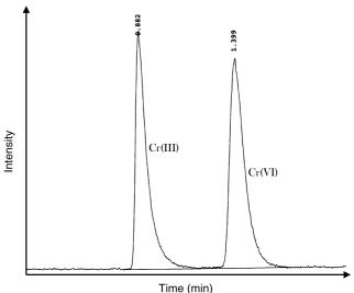
**Figure 3** Typical chromatogram achieved using the 3 mM  $HCO_3^-$ , 9 mM  $CO_3^{-2}$  and 5 mM EDTA eluent (sample: 20 mg  $L^{-1}$  Cr(III) and 20 mg  $L^{-1}$
