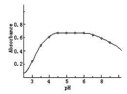
**Figure 6** Effect of pH on the formation of Co(II) complex, Co(II) concentration was  $5.0 \times 10^{-6}$  mol L<sup>-1</sup>, other conditions as general procedure.
