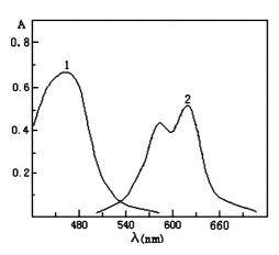
**Figure 5** Absorption spectra of QADMAA and its Co(II) complex: (1) QADMAA-CTMAB blank against water; (2) QADMAA-Co(II)-CTMAB complex against reagent blank.
