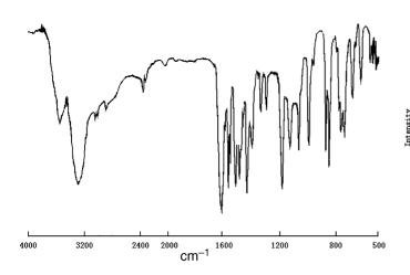
Figure 1 The infrared spectrum of QADMAA.
