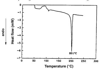
Figure 1 DSC trace of the pure alcohol host 4.
