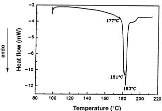
Figure 3 DSC trace for the  $4 \cdot DMSO$  enclathration complex (heating rate: 2.5 K min<sup>-1</sup>).
