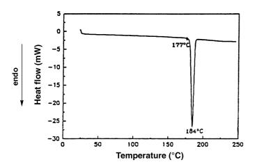
Figure 2 DSC trace for the  $4\cdot DMSO$  enclathration complex (heating rate:  $5\,K\,min^{-1}).$
