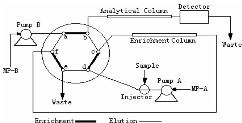
**Figure 1** On-line enrichment system using the valve-switching technique. Pump A, Waters 515 Pump. Pump B, Waters 2690 Alliance quadripump. Injector can contain a 10 mL sample. Six-port switching valve (Waters Corporation). Enrichment Column, ZORBAX (4.6 × 10 mm, 1.8 μm). Analytical column, ZORBAX (4.6 × solution. MP B, 72% methanol (containing 0.05 mol L<sup>-1</sup> of pH = 3.8 sodium acetate-acetic acid buffer salt and 0.1% of triton X-100).
