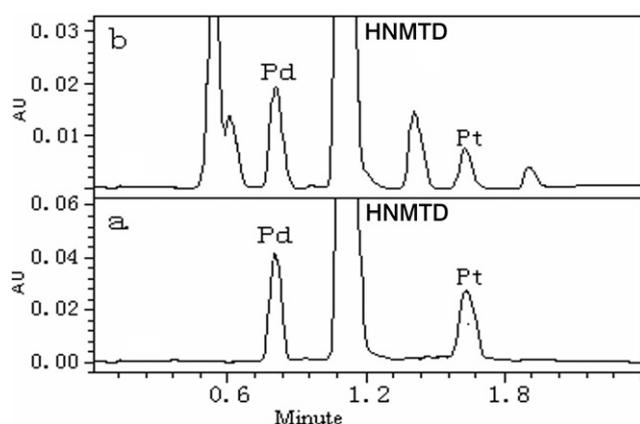
**Figure 2** Chromatogram of (a) standard sample and (b) occupationally exposed human urine samples. The concentration of palladium and platinum is  $1.0 \mu\text{g L}^{-1}$  in standard sample, and the other conditions are as in the standard procedure.
