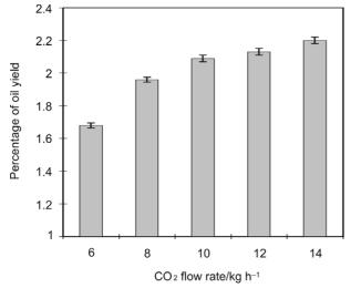
Fig. 4 Effect of CO<sub>2</sub> flow rate.
