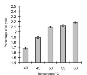
Fig. 3 Effect of extraction temperature.
