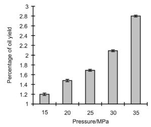
Fig. 2 Effect of extraction pressure.
