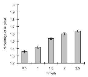
Fig. 1 Effect of extraction time.
