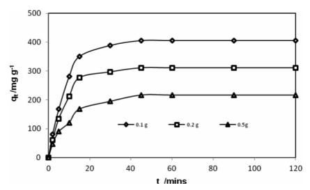
Figure 2 Effect of adsorbent dosage on the adsorption of MG dye by OPFAC (Conditions:  $100 \text{ mg L}^{-1}$ , pH 6, 120 rpm, 120 min agitation time temperature  $30 \,^{\circ}\text{C}$ ).
