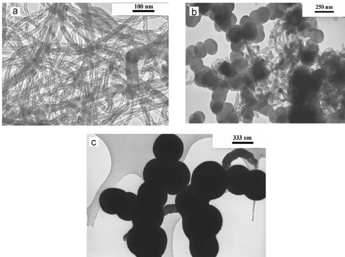
**Figure 7** Low magnification TEM images of the carbon deposit produced with different dilution ratios of feedstock gases: (a)  $C_2H_2:N_2 = 1:2.7$  (100 % CNTs), (b)  $C_2H_2:N_2 = 1:1$  (CNTs and CMSs), (c) pure  $C_2H_2$  (CMSs and CNFs);  $T = 700\text{ }^\circ\text{C}$ ,  $t = 1\text{ h}$ .
