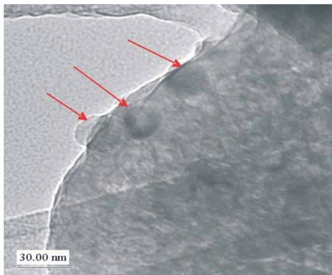
**Figure 3** TEM image of IMPN. Arrows show some Fe-Co nanoparticles (~30 nm) supported on CaCO<sub>3</sub> after calcination.
