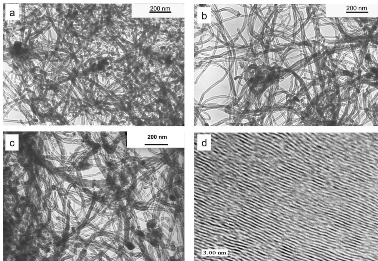
**Figure 4** TEM images of MWCNTs prepared by the (a) IMPN, (b) DPN, (c) RM methods and (d) a general higher magnification TEM image showing a much closer look at the 'wavy-like' 0.34 nm (0002) graphite lattice fringes of the CNTs.
