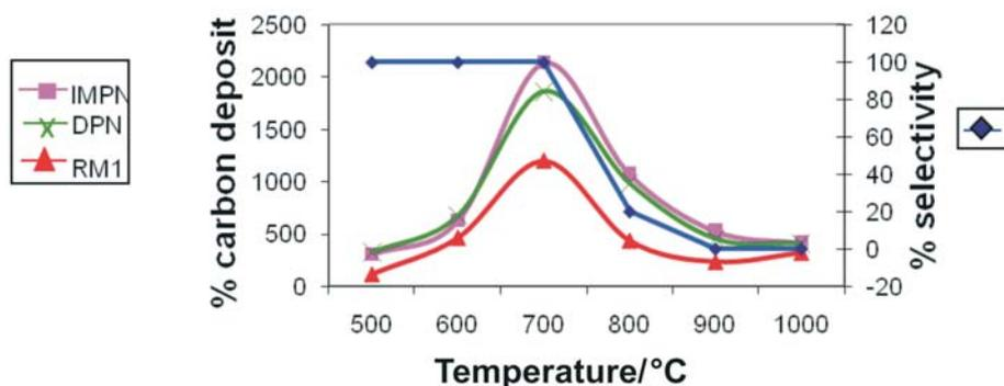
**Figure 5** Graph showing the amount of CNTs produced and the percentage selectivity at different reaction temperatures in the CVD of  $C_2H_2$  diluted with  $N_2$  ( $C_2H_2:N_2 = 1:3$ ,  $t = 1$  h). The selectivity profile is similar for all the supported catalysts.
