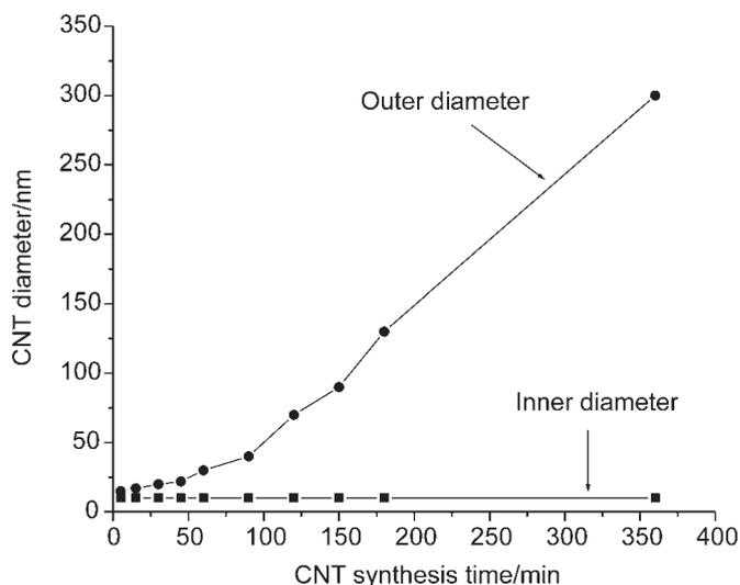
**Figure 10** A plot of variation of the CNT diameter with time for CNTs synthesized over IMP Fe-Co/CaCO<sub>3</sub> catalysts.
