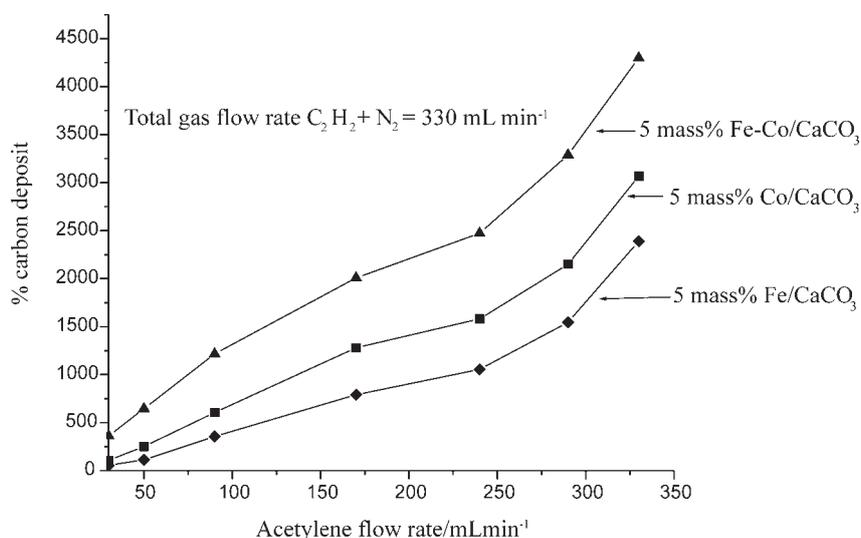
**Figure 6** A graph showing percentage C obtained by varying the gas flow ratio of  $C_2H_2$  to  $N_2$ . The synthesis time was 1 h for all reactions and the reaction temperature was 700 °C.
