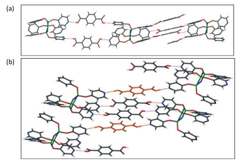
Figure 3 (a) The infinite hydrogen-bonded chain formed in 7°TPA. (b) The hydrogen-bonded chains are linked *via* a terephthalic acid molecule, shown here in orange, that hydrogen bonds to the pyridyloxy group of a neighbouring cyclotriphosphazene molecule.
