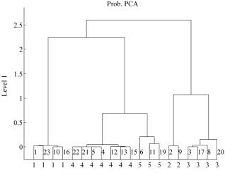
**Figure 6** Dendogram of South African clinkers constructed from the two-dimensional latent variables. The *y*-axis shows the distances between clusters. Numbers at the bottom are the factory codes, while numbers within the dendrogram are the sample codes.
