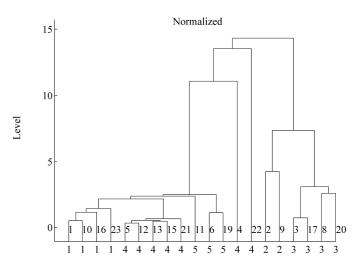
**Figure 2** Dendogram of South African clinkers constructed from normalized data. The *y*-axis shows the distances between clusters. Numbers at the bottom are the factory codes, while numbers within the dendrogram are the sample codes.
