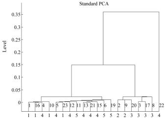
**Figure 4** Dendogram of South African clinkers constructed from data projected into the first two principal components. The *y*-axis shows the distances between clusters. Numbers at the bottom are the factory codes, while numbers within the dendrogram are the sample codes.
