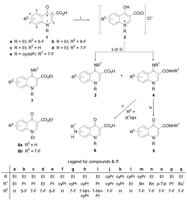
**Scheme 1** Reagents and conditions: i, SOCl<sub>2</sub>, reflux; ii,  $R^1NH_2 + H_2O (\rightarrow 3 > 4)$ ; iii, dry  $R^1NH_2 (\rightarrow 4 > 3)$ ; iv, NMe<sub>4</sub>OH–H<sub>2</sub>O, reflux; v, aq. NaOH, reflux. The geometry of the imines depicted above and elsewhere is not specified.
