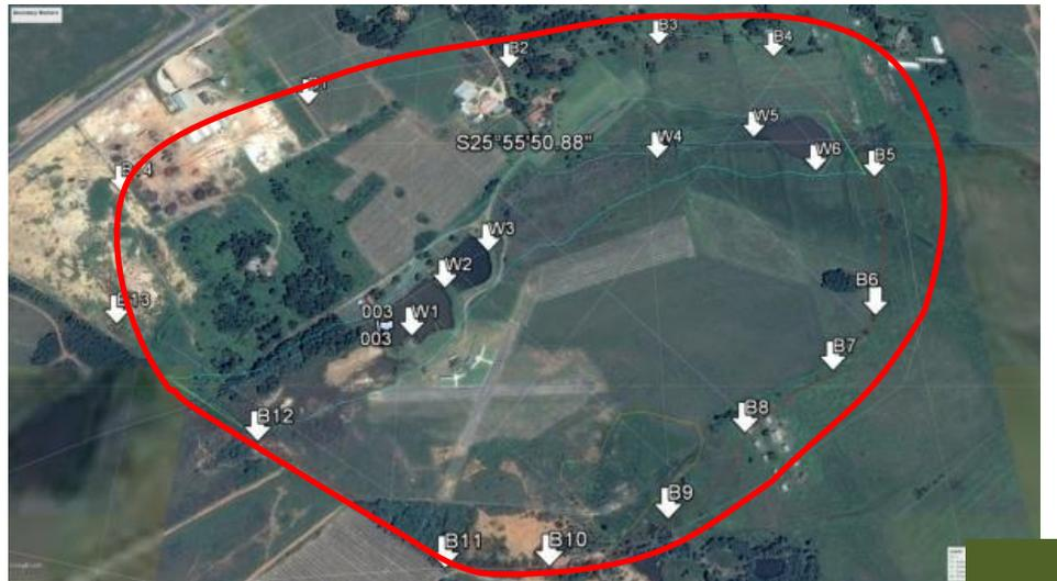
Figure 3. Ground control markers (arrows) positioned at the boundaries of the UAV survey area/study area (red line) including next to the watercourse at different elevations
