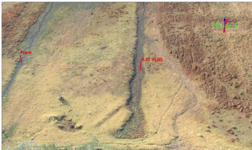
Figure 7. The 0.38m 3D dense point cloud allows accurate measurement of depth of drains within the wetland
