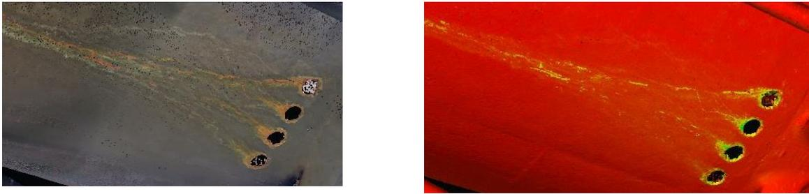
Figure 15 (left). True colour point cloud of the drainage pattern of corrosion on the keel of a vessel
