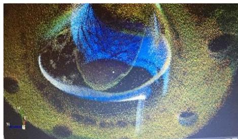
Figure 8. a 3D visual of corrosion in a CAD package, nodes of accretion and wear pattern is observable
