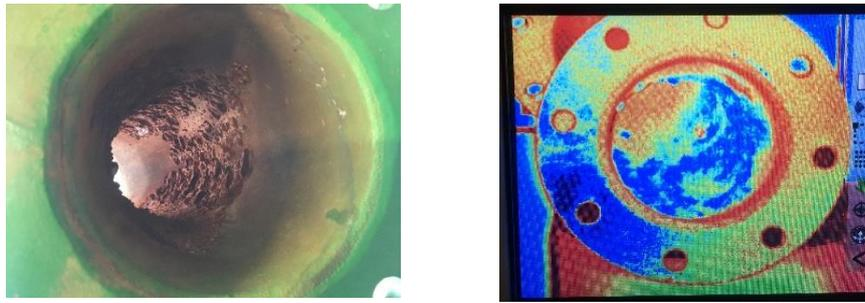
Figure 6 (left). Internal corrosion on a mine pipe
