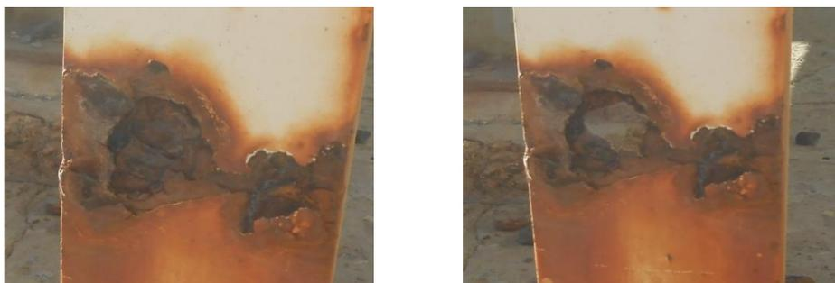
Figure 2 (left). Localized corrosion before the corrosion products have been removed
