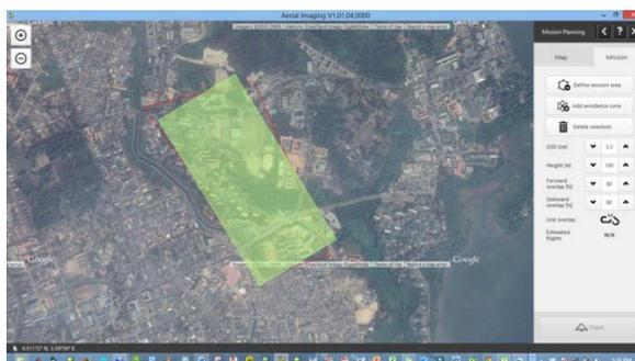
Figure 3. Trimble Access Aerial Imaging Software showing the desired GSD, flying height and Overlap
