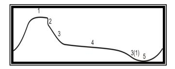
Figure 3: Terrain units, where 1 represents a crest, 2 a scarp, 3 a mid-slope, 3(1) a secondary midslope, 4 a foot-slope and 5 a valley.
