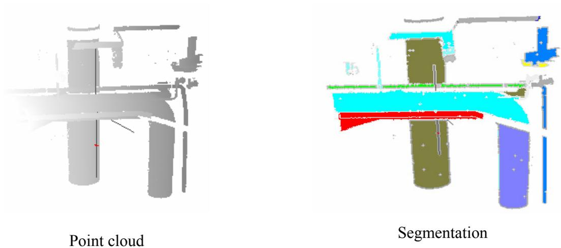
Figure 12. Segmentation of a piping installation.
