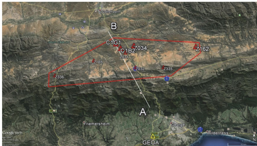
Figure 1. Blossoms wellfield and far-field boreholes (within the red polygon) relative to Oudtshoorn, George and the TrigNet station GEOA. Some boreholes are not shown for clarity. GNSS receivers were located at boreholes C1B2, C1G1, Z034 and Z162 for 133 days. C1B2 is approximately 25 m NW of C1B3. The polygon is approximately 50 km by 11 km in extent. The line AB represents the geological profile in Figure 2.
