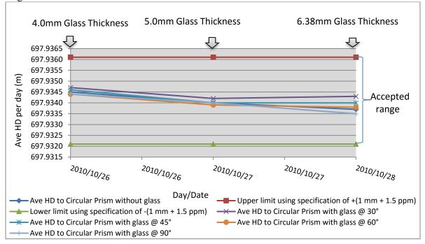
Figure 6: Average HDs to circular prism corrected for prism constant, scale factor, atmospheric and glass thickness, as seen in the second target station
