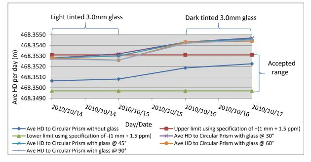
Figure 7: Average HDs to circular prism corrected for prism constant, scale factor and atmospheric corrections, but not corrected for glass thickness impact, as seen in the first target station
