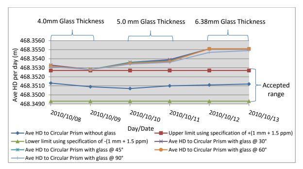
Figure 3: Average HDs to circular prism corrected for prism constant, scale factor and atmospheric corrections, but not corrected for glass thickness impact, as seen in the first target station
