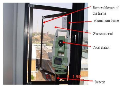
Figure 1: Instrument station set-up showing window frame, total station and beacon
