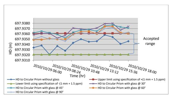
Figure 9: HDs to circular prism after prism constant, scale factor and atmospheric corrections, but before glass colour correction using light tinted 3.0mm glass, as seen in the second target station
