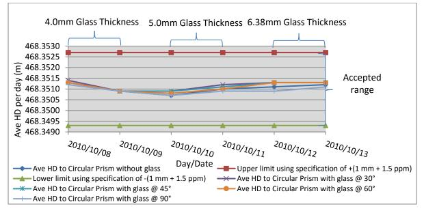
Figure 4: Average HDs to circular prism corrected for prism constant, scale factor, atmospheric and glass thickness, as seen in the first target station
