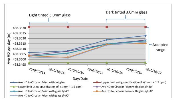
Figure 8: Average HDs to circular prism corrected for prism constant, scale factor, atmospheric and glass thickness, as seen in the first target station
