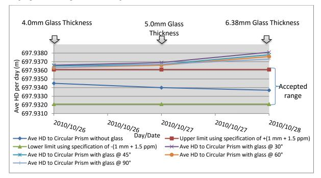
Figure 5: Average HDs to circular prism corrected for prism constant, scale factor and atmospheric corrections, but not corrected for glass thickness impact, as seen in the second target station
