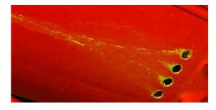
Figure 15 (left). True colour point cloud of the drainage pattern of corrosion on the keel of a vessel Figure 16 (right). Keel corrosion pattern in RGB values
