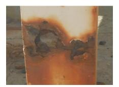
Figure 2 (left). Localized corrosion before the corrosion products have been removed Figure 3 (right). Localized corrosion after removal of the corrosion products the severity of the damage is evident
