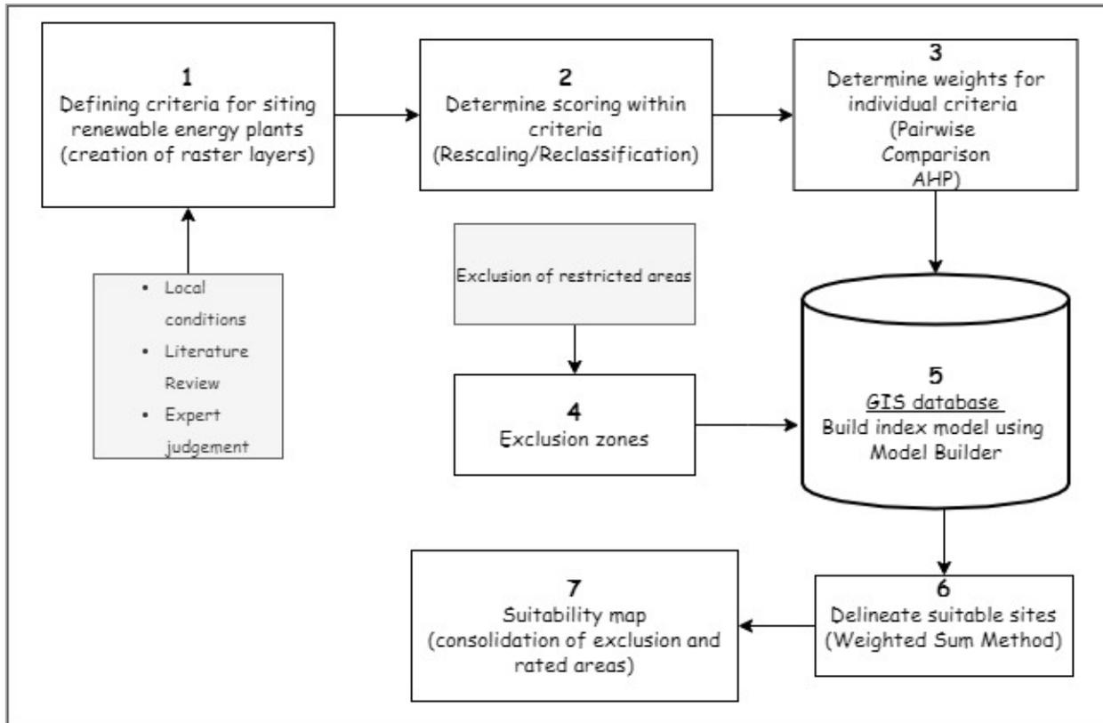
Figure 1: Methodological framework for siting wind, solar and small hydro power plants
