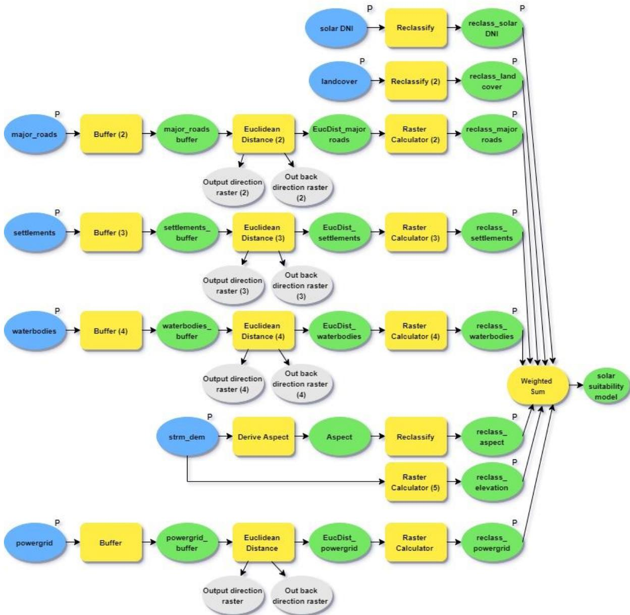
Figure 3: Illustration of GIS index model for solar suitability constructed using Model Builder
