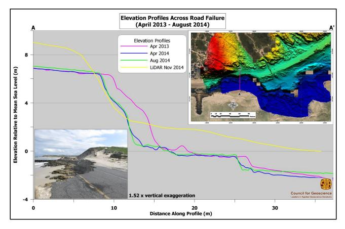
Figure 3. Comparison of the different elevation profiles across the road failure. Top right inset map reflects relative position of transect within the study area (magenta line). Bottom left is a picture courtesy of W. Van Zyl of the failed road.
