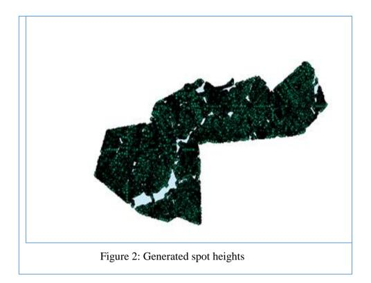
The Natural neighbor interpolation tool in spatial analyst toolbox was used to interpolate and convert the random points obtained from the contour map into a gridded surface raster. The leveled spot heights coverage of the area was overlaid on the raster surface map to enable corresponding values from the surface map to be extracted to points. As such, values from each surface matching point were extracted with its matching values from the leveled dataset.
