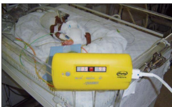
The wind-up pulse oximeter being used to measure the oxygen saturation of a preterm infant with respiratory distress receiving continuous positive airway pressure support.
