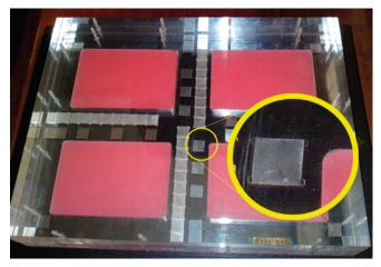
Fig. 1. The APG phantom used for MTF evaluation. The enlarged area shows an MTF plate.
