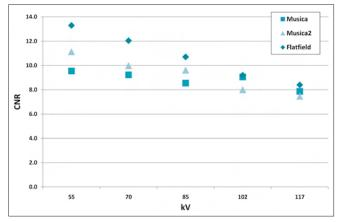
Fig. 3. Average contrast-to-noise ratios calculated from steps 1 to 4 of the step wedge at all energies.
