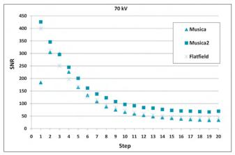
Fig. 2. Signal-to-noise ratios for all steps imaged at 70 kV. Readout artefacts can cause outliers as seen at step 1 (MUSICA).
