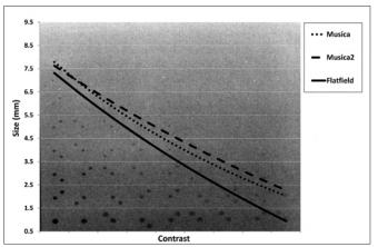
Fig. 4. Graph showing contrast with decreasing object size for the different algorithms.
