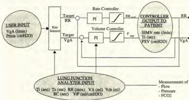
Fig. 1. Diagram of the ALV controller showing the input and output relationships. User input is  $V'gA$  (l/min) and  $P_{max}$  (cm  $H_2O$ ). Lung function analyser input is  $T_i$  (s),  $T_e$  (s),  $RR$  (/min),  $V_A$  (ml),  $V_{ds}$  (ml),  $RC$  (s) and  $V/P$  ratio (ml/cm  $H_2O$ ). Controller output is mandatory rate (/min),  $T_i$  (s) and  $P_{insp}$  (cm  $H_2O$ ). (From *Chest*.<sup>3</sup>)
