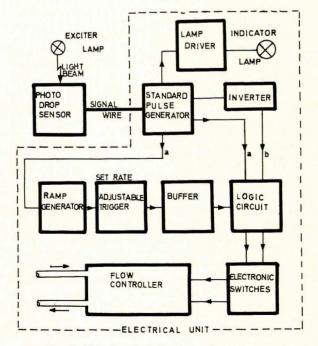
Fig. 2. The electrical elements of the system.
