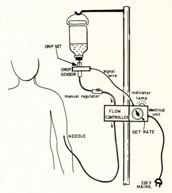
Fig. 1. The physical layout of the system.
