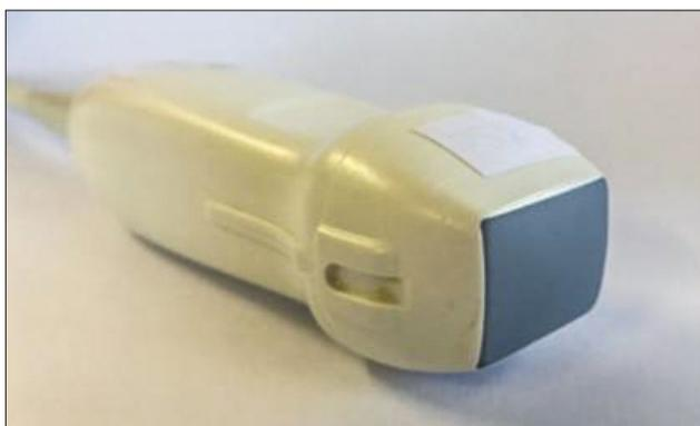
Fig. 1. Phased-array probe.
