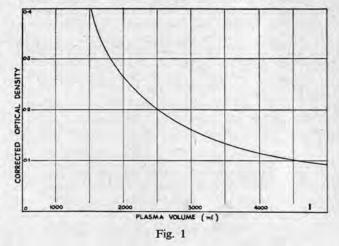
optical densities were read on a Beckman DU Spectrophotometer at 620 m $\mu$ . The data thus obtained were used for the construction of a standard curve (Fig. 1). The curve was found to be a hyperbola which could be represented by the equation:
