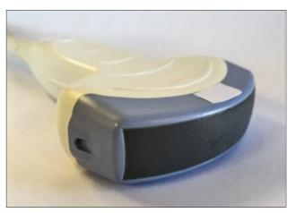
Fig. 2. Curvilinear probe.
