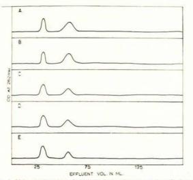
Fig. 3. Urinary albumins of the cadmium-poisoned monkey G. following a pulse dose of 6 mg. cadmium given intravenously. A - E = 1-5 days respectively after the dose. Albumins prepared and separated as in Fig. 1. Column 25 x 2.5 cm. Flow rate = 18 mL/hr. OD recorded at 262 m<sub>µ</sub>.
