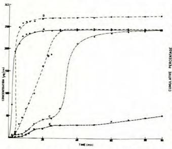
Fig. 3. Dissolution rate of chloramphenicol in different capsules.
