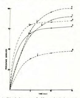
Fig. 1. Dissolution rate of chloramphenicol capsules as determined with disintegration apparatus. Arrows indicate disintegration time.
