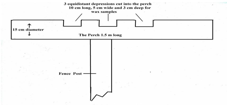
Figure 1. The perch diagrammatically and not to scale.
