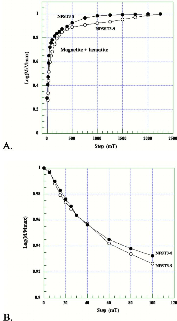
Figure 2. (A) IRM acquisition experiment for representative specimens from Enticho Sandstone at Negash. (B) AF demagnetization curve of the IRM experiment in A; the corresponding specimen names are given.
