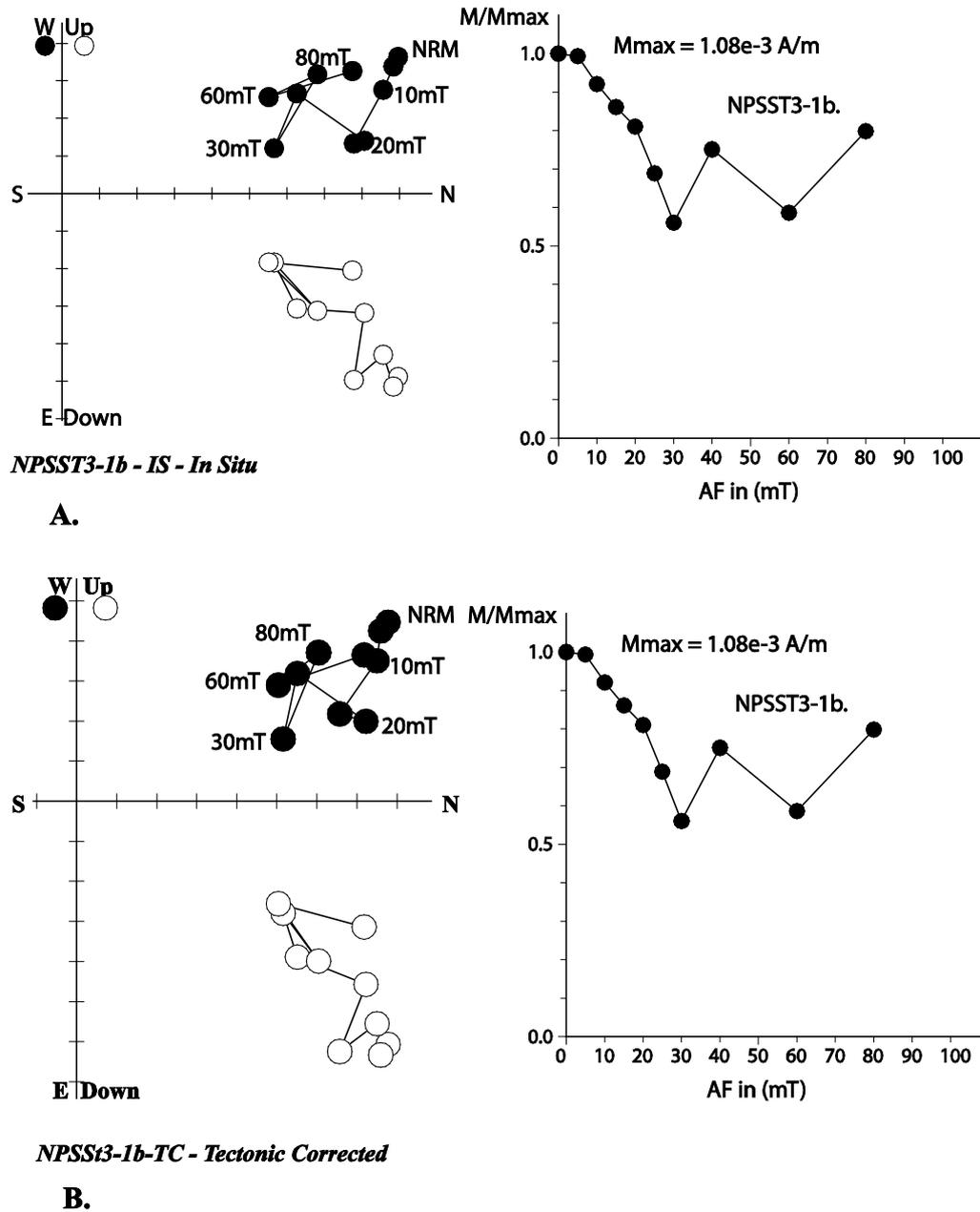
Figures 3 A and B. Examples of Zijderveld diagrams for specimens from the Enticho Sandstone at Negash area one treated by Alternating Field (AF) and another by thermal demagnetization techniques. A represents the *in-situ* coordinate; B represents the tectonic corrected coordinates. (The magnetic polarity is down and pointing north consistent with normal configuration for the location).
