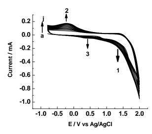
Fig. 1. Repetitive cyclic voltammograms (a-j) of  $2.0 \times 10^{-3}$  mol L<sup>-1</sup> para-aminosalicylic acid in 0.1M HNO<sub>3</sub> at the MWCNTS/GCE. Scan rate: 100 mV s<sup>-1</sup>.
