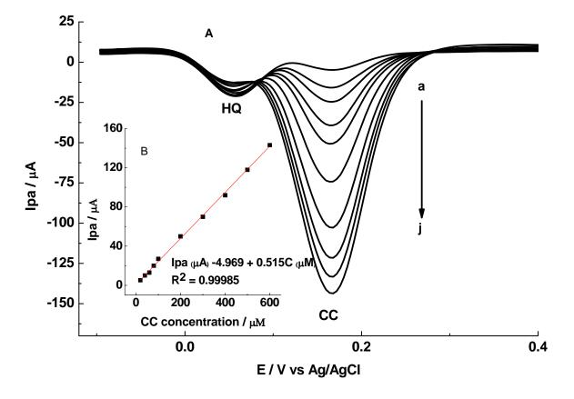
Fig. 7. (A) DPVs of poly(p-ASA)/MWCNTs/GCE in a binary mixture of variable concentration of CC and constant concentration of HQ in pH 7.0 PBS (a → j: 20, 40, 60, 80, 100, 200, 300, 400, 500 and 600 × 10<sup>-6</sup> mol L<sup>-1</sup> of CC and 1 × 10<sup>-4</sup> mol L<sup>-1</sup> HQ);
