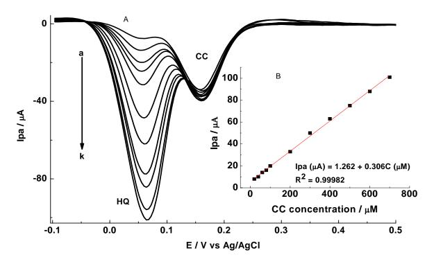
Fig. 6. (A) DPVs of poly(p-ASA)/MWCNT5/GCE in a binary mixture of variable concentration of HQ and constant concentration of CC in pH 7.0 PBS (a→k: 20, 40, 60, 80, 100, 200, 300, 400, 500, 600 and 700×10<sup>-6</sup> mol L<sup>-1</sup> of HQ and 1×10<sup>-4</sup> mol L<sup>-1</sup> CC);
