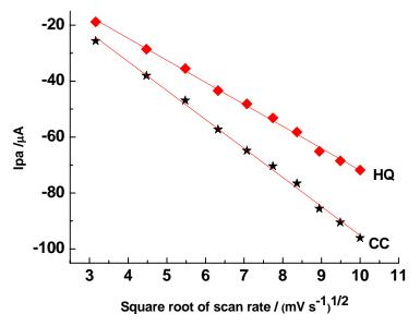
Fig. 4. Oxidative peak current vs square root of scan rate curve of 1 × 10-3 mol L-1 CC and HQ in the range of 10 to 100 mV s-1.
