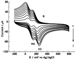
Fig. 3B Cyclic voltammograms of  $1 \times 10^{-3}$  mol L<sup>-1</sup> HQ and CC in pH 7.0 PBS at Poly(p-ASA)/MWCNTS/GCE at different scan rates (a  $\rightarrow$  j: 10, 20, 30, 40, 50, 60, 70, 80, 90 and 100 mV s<sup>-1</sup>).
