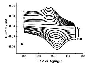
Fig. 2B. Cyclic voltammograms of poly(p-ASA)/ MWCNTs/ GCE in pH 7 PBS at different scan rates ( from inner to outer waves: 50, 100, 150, 200, 250, 300, 350, 400, 450, 500, 550 and 600 mV s<sup>-1</sup>).
