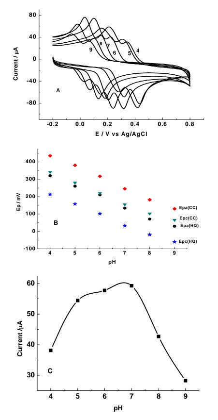
Fig. 5. (A) Cyclic voltammograms of poly(p-ASA)/MWCNTs/GCE in different pHs of 0.1 M PBS containing binary mixture of CC and HQ (each 1×10<sup>-3</sup> mol L<sup>-1</sup>); (B) Plot of Ep vs pH of buffer solution; (C) The effect of pH of the solution on the anodic peak current of CC in a binary mixture of CC and HQ. pH range 4.0-9.0; scan rate: 0.1 Vs<sup>-1</sup>; sensitivity: 100 µA V<sup>-1</sup>.
