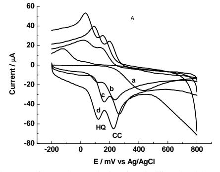
Fig. 3A. Cyclic voltammograms of 1 × 10<sup>-3</sup> mol L<sup>-1</sup> HQ and CC in PBS (pH 7.0) at different electrodes: bare GCE (a), poly(p-ASA)/GCE (b), MWCNTs/GCE (c) and poly(p-ASA)/ MWCNTs/GCE (d). Scan rate: 20 mV s<sup>-1</sup>.
