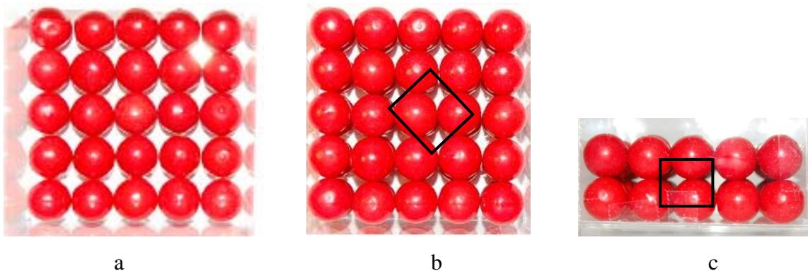
Figure 1. Simple cube model. a) top view of the first layer, b) top view of the first two layers, c) side view of the two layers.
