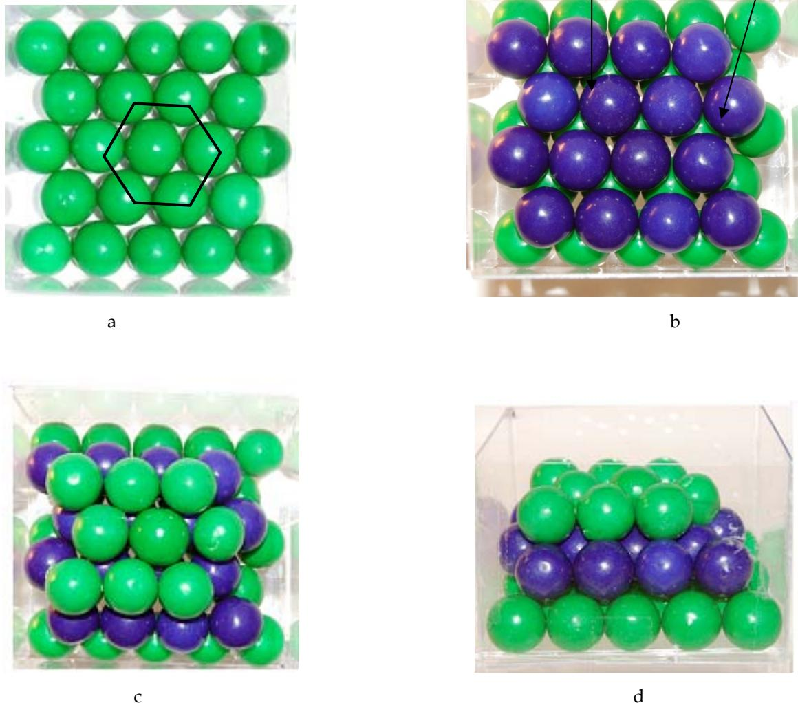
Figure 3. Hexagonal close-packing model. a) top view of the first layer of hexagonal packing, b) top view of the first two layers, c) top view of three ABAB... layers, d) side view of ABAB... layer.
