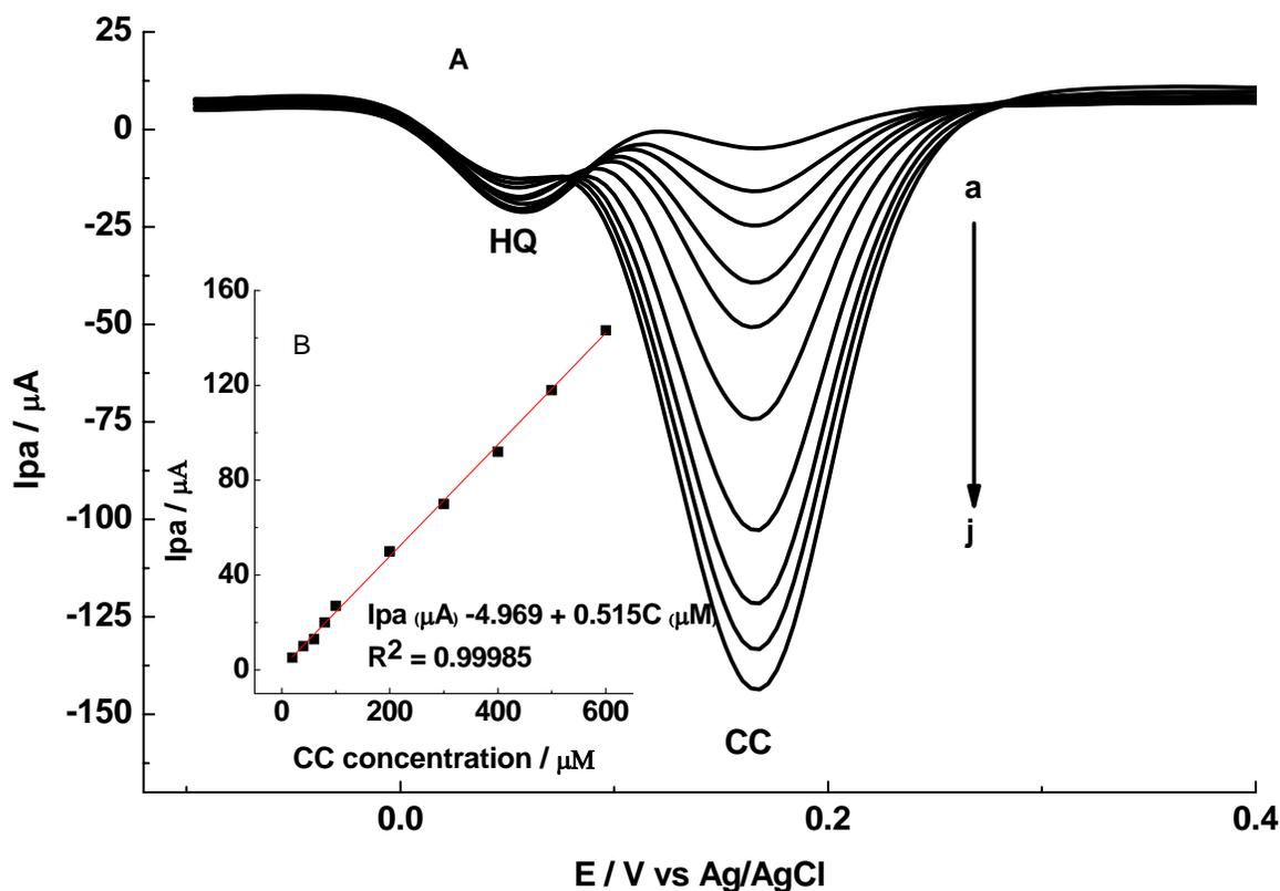
Fig. 7. (A) DPVs of poly(p-ASA)/MWCNTs/GCE in a binary mixture of variable concentration of CC and constant concentration of HQ in pH 7.0 PBS (a  $\rightarrow$  j: 20, 40, 60, 80, 100, 200, 300, 400, 500 and 600  $\times 10^{-6}$  mol L<sup>-1</sup> of CC and  $1 \times 10^{-4}$  mol L<sup>-1</sup> HQ); (B) plot of anodic peak current of CC at the modified GCE vs concentration. Scan rate: 50 mV s<sup>-1</sup>; pulse amplitude: 20 mV.
