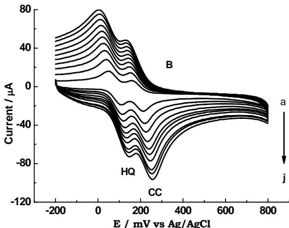
Fig. 3B Cyclic voltammograms of  $1 \times 10^{-3}$  mol L<sup>-1</sup> HQ and CC in pH 7.0 PBS at Poly(p-ASA)/MWCNTs/GCE at different scan rates (a → j: 10, 20, 30, 40, 50, 60, 70, 80, 90 and 100 mV s<sup>-1</sup>).
