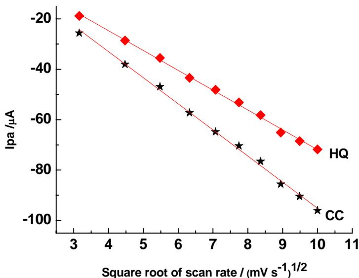
Fig. 4. Oxidative peak current vs square root of scan rate curve of  $1 \times 10^{-3}$  mol L<sup>-1</sup> CC and HQ in the range of 10 to 100 mV s<sup>-1</sup>.
