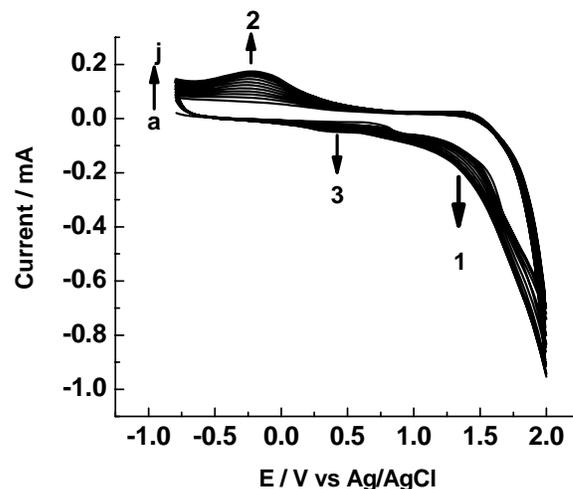
Fig. 1. Repetitive cyclic voltammograms (a-j) of 2.0 × 10<sup>-3</sup> mol L<sup>-1</sup> *para*-aminosalicylic acid in 0.1M HNO<sub>3</sub> at the MWCNTs/GCE. Scan rate: 100 mV s<sup>-1</sup>.
