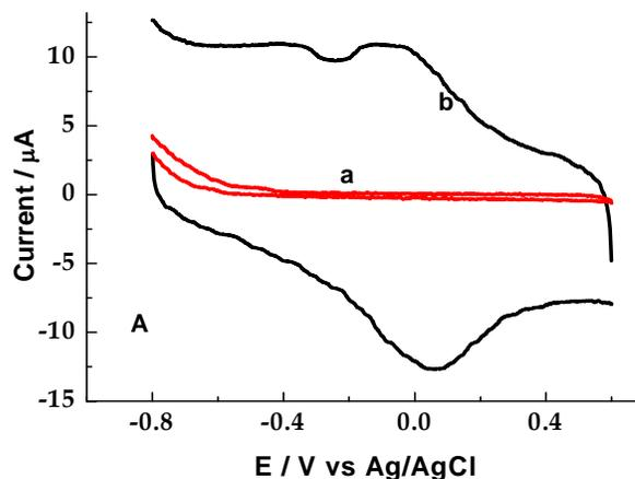
Fig. 2A. Cyclic voltammogram of bare GCE (a) and stabilized poly(p-ASA)/MWCNTs/GCE (b) in pH 7 PBS at a scan rate of 0.1 V s<sup>-1</sup>.
