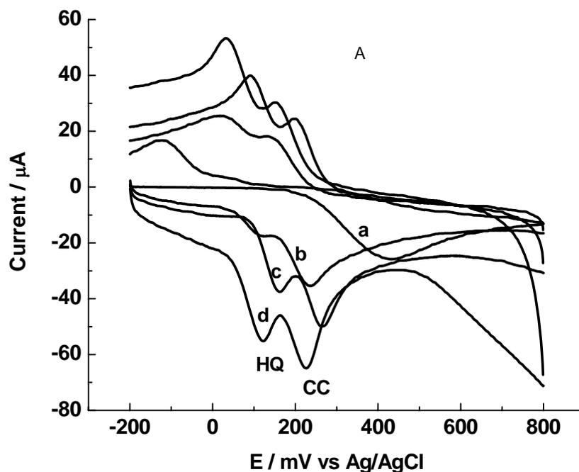
Fig. 3A. Cyclic voltammograms of  $1 \times 10^{-3}$  mol L<sup>-1</sup> HQ and CC in PBS (pH 7.0) at different electrodes: bare GCE (a), poly(p-ASA)/GCE (b), MWCNTs/GCE (c) and poly(p-ASA)/MWCNTs/GCE (d). Scan rate: 20 mV s<sup>-1</sup>.
