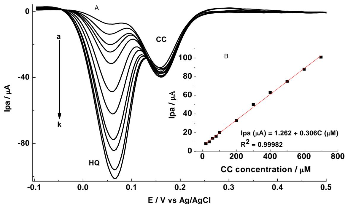
Fig. 6. (A) DPVs of poly(p-ASA)/MWCNTs/GCE in a binary mixture of variable concentration of HQ and constant concentration of CC in pH 7.0 PBS (a → k: 20, 40, 60, 80, 100, 200, 300, 400, 500, 600 and  $700 \times 10^{-6}$  mol L<sup>-1</sup> of HQ and  $1 \times 10^{-4}$  mol L<sup>-1</sup> CC); (B) plot of anodic peak current of HQ at the modified electrode vs concentration. Scan rate: 50 mV s<sup>-1</sup>; pulse amplitude: 20 mV.
