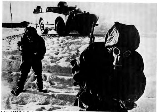
A Soviet BRDM-rkh Radiological-Chemical Reconnaissance vehicle with area warning emplacers. The vehicle explores the boundaries of an infected zone and marks the limits.
