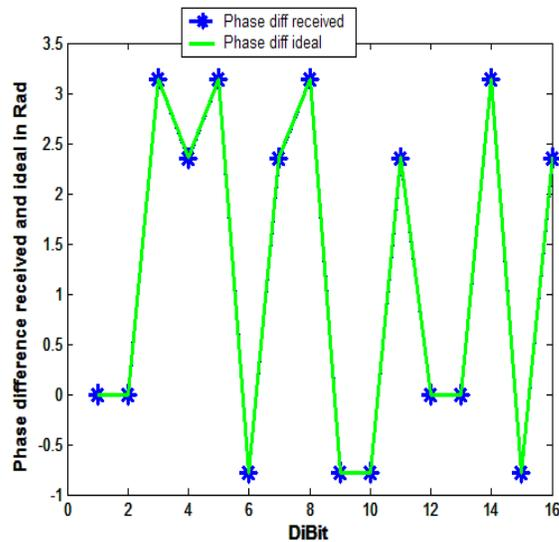
**Figure 7.** Phase comparison between the expected and received phase differences for SMF fiber link with MSS1 compensation used in the presence of the nonlinear effect.
