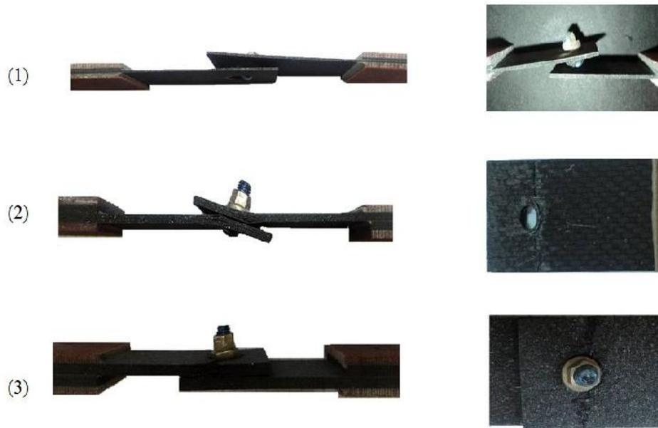
Figure.7. Macroscopic view of post-mortem; (1) specimen A, (2) specimen B, (3) specimen C.
