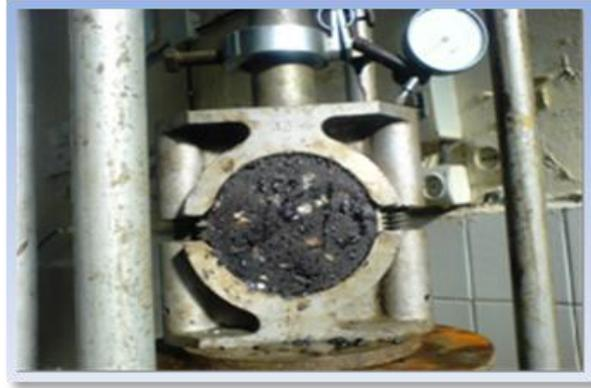
Figure 5. Marshall Test
