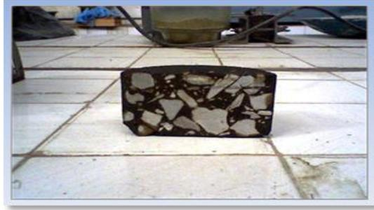
Figure 7. Specimens after storage 48 h in the oven.(Filler 10%)
