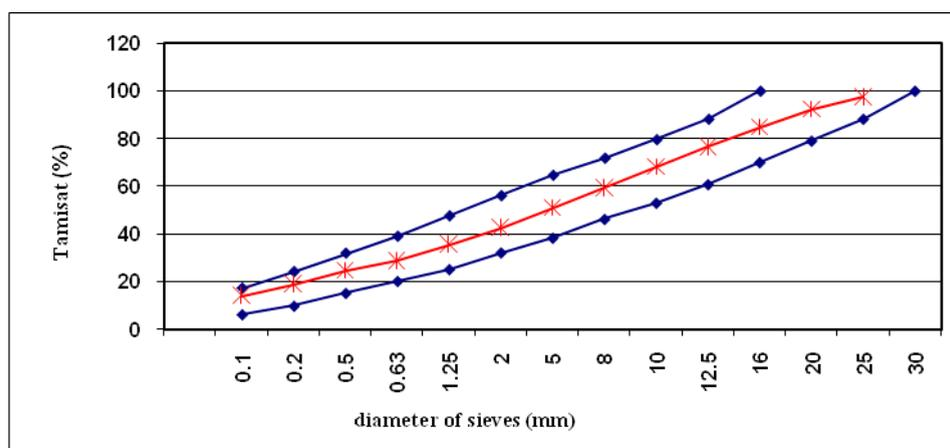
Figure 3.c. Grading curve of the 3rd mixture « Filler 20 % »
