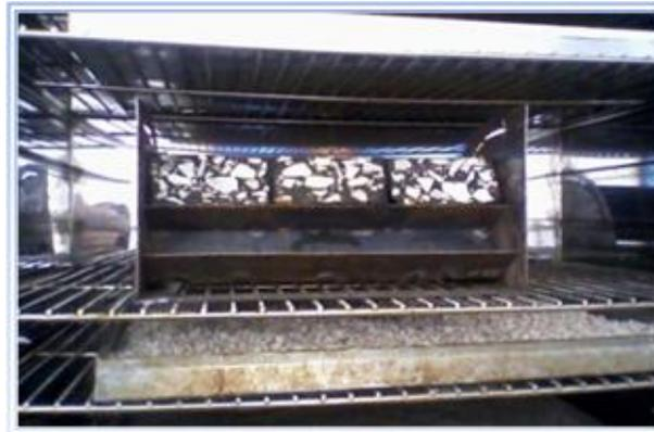
Figure 6. Preserved test-tubes 48h in the drying oven
