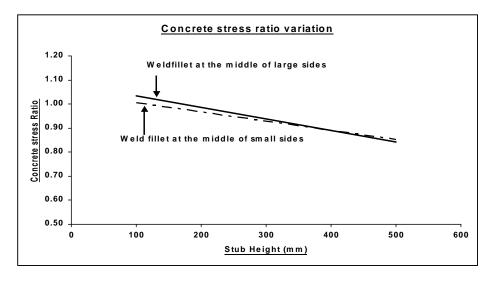
Figure 4. Concrete mean stress ratio as a function of stub height.
