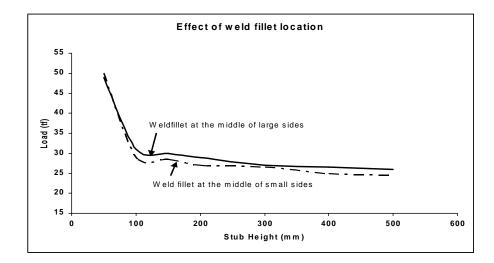
*Figure 3. Experimental failure loads for composite tubes with different weld fillet locations.*
