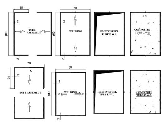
Figure 1. Manufactured steel and composite cross section beams.
