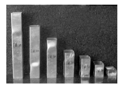
Figure 6. Empty steel stubs EWL after test.
