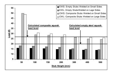
Figure 5. Experimental failure loads comparison.
