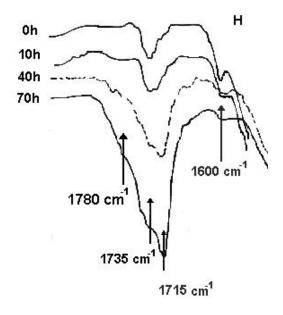
*Figure 5. IR* spectra of stabilized [PVC H, DLS] for three aging stages (carbonyls region).
