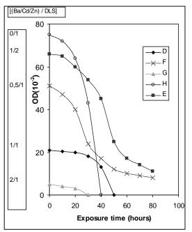
*Figure 9.* Variation of the carboxylate metal salts absorption at  $(1510-1540 \text{ cm}^{-1})$  vs. time exposure
