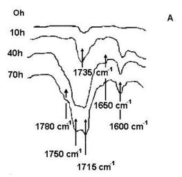
*Figure 3. IR* spectra [*PVC* (*A*), (*Unstabilized*)] for three aging stages (carbonyls region).
