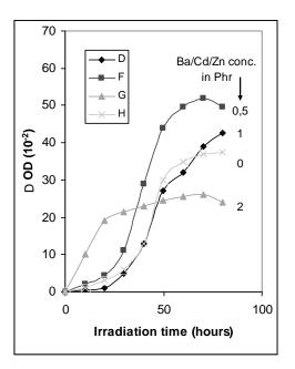
*Figure 8. Relative optical density at 1715 cm<sup>-1</sup> vs. exposure time (effect of Ba/Cd/Zn added to 1Phr of DLS).*
