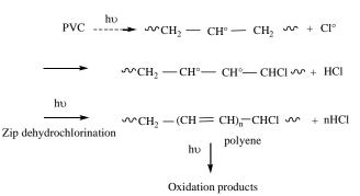
*Figure 1. Zip dehydrochlorination mechanism.*
