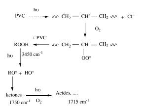
*Figure 2. Simplified mechanism of PVC photo-oxidation.*
