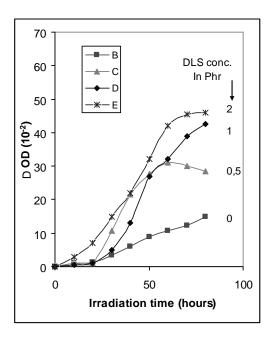
*Figure 7. Relative optical density at 1715* cm<sup>-1</sup> vs. *exposure time (effect of DLS added to 1Phr of Ba/Cd/Zn).*
