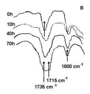
*Figure 4. IR* spectra of stabilized [PVC B, (Ba/Cd/Zn)] for three aging stages (carbonyls region).
