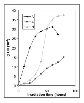
**Figure 6.** Relative optical density at 1715  $cm^{-1}$  vs exposure time, PVC A, B and H, effect of the respective stabilizers on the oxidation kinetic.
