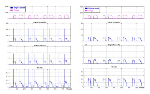
Figure 5 : PID controller simulation results in urban driving cycle (UDC standards).
