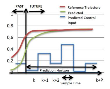
Figure 3 : A discrete MPC scheme.
