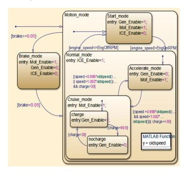
Figure 9 : Mode logic modelled with Stateflow®.
