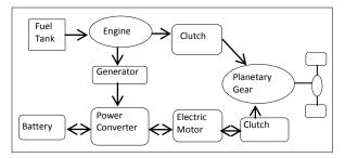
Figure 1 : Structure of series-parallel HEV.
