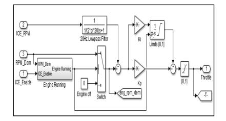
Figure 4 : Engine speed controller.
