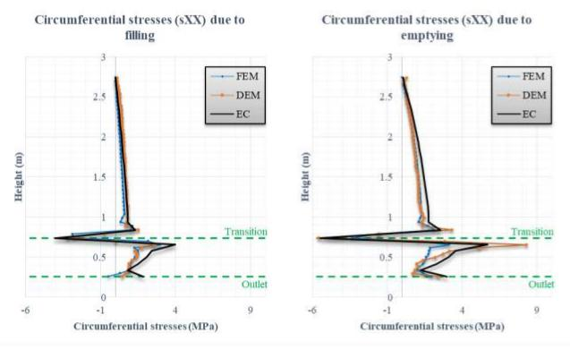
**Figure 7.** The values of the circumferential stresses in the silo walls due to filling and emptying by the FEM, DEM, and EC.
