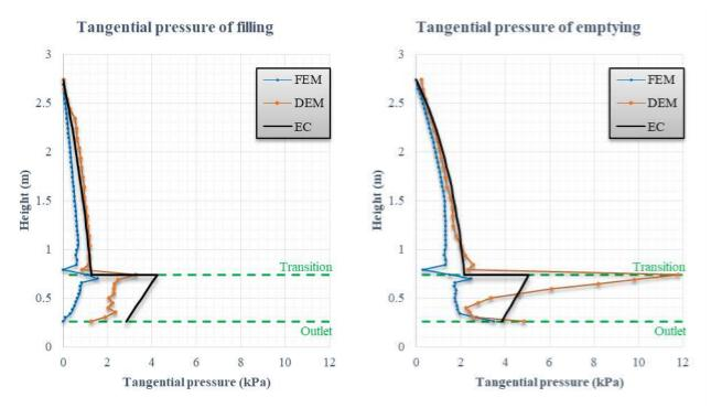
Figure 6. The values of the tangential pressures in the silo walls due to filling and emptying by the FEM, DEM, and EC.
