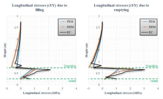
Figure 8. The values of the longitudinal stresses in the silo walls due to filling and emptying by the FEM, DEM, and EC.
