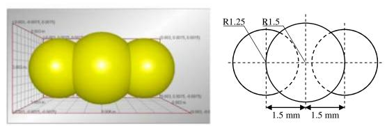
Figure 3. Particle model of the wheat grain.
