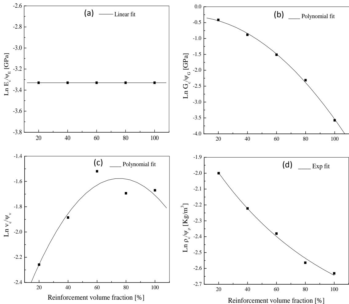
Figure 3. Vit.1 matrix composites slopes curves of fig. 2 variations as function of reinforcement volume fraction.
