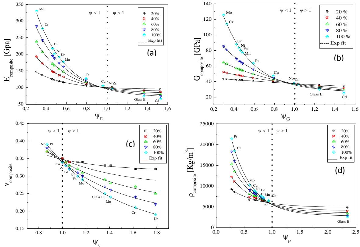
Figure 2. Vit.1 matrix composites mechanical properties variations as function of  $\psi$  ratio for various reinforcement volume fractions.(a) Young's modulus, (b) shear modulus, (c) Poisson ratio & (d) density.
