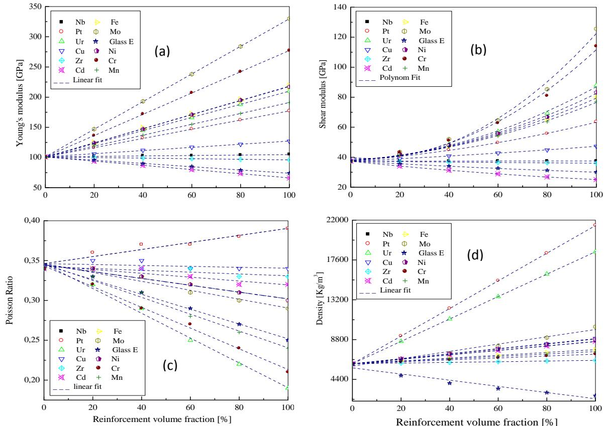
Figure 1. Vit.1 matrix composites density & elastic constants as function of reinforcement volume fraction of , glass E, Fe, Mo, Ni, Cr, Mn, Nb, Cd, Pt, U, Zr: (a) Young's modulus, (b) shear modulus, (c) Poisson ratio & (d) density.
