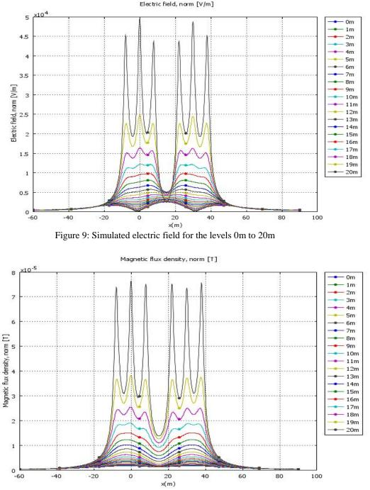
Figure 10: Simulated magnetic fields for the levels 0m to 20m
