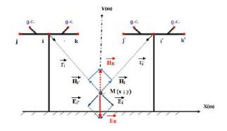
Figure 4: Analytical model for EMF calculation
