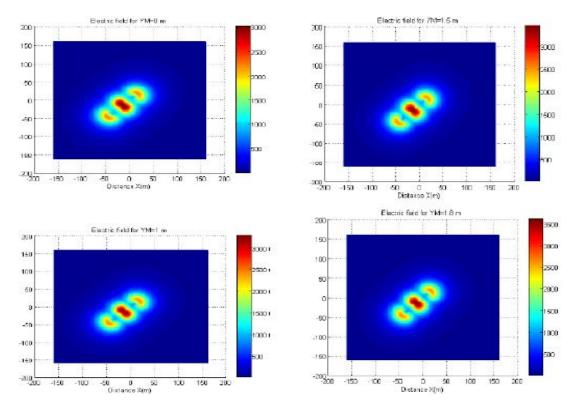
Figure 6: Electrical field distribution, plane X-Y, for 4 levels (0m, 1m, 1.5m and 1.8m ©UBMA - 2015
