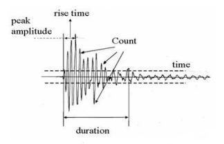
Figure.4: Parameters of acoustic emission.
