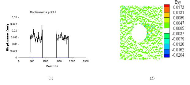
Figure.12: (1). Field of displacement at point d along line (z), (2) the strain field at point d.
