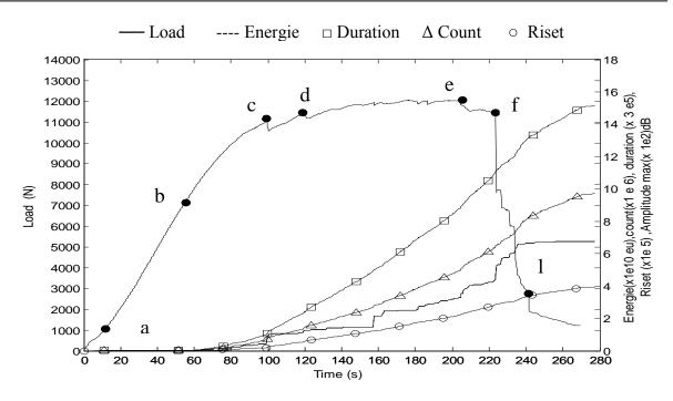
Figure.9 Load applied against time of the specimen C followed by the acoustic parameters as energy cumulated count number the energy, duration of the signal and rise.
