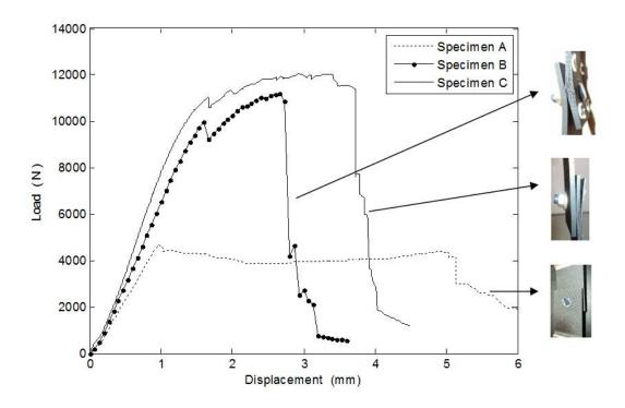
Figure.6: Loading function displacement of the three types of test specimen
