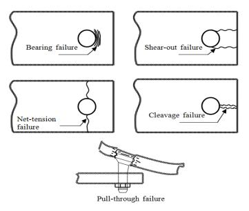
Figure.1: Failure modes of a bolt loaded hole.
