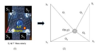
Figure.5. (1) location of acoustic output source, (2) Sensors and acoustic source position for 4 channel position, O(x,y) acoustic source position, and  $O_1$ ,  $O_2$ ,  $O_3$ ,  $O_4$  represent the sensor-to-source distances
