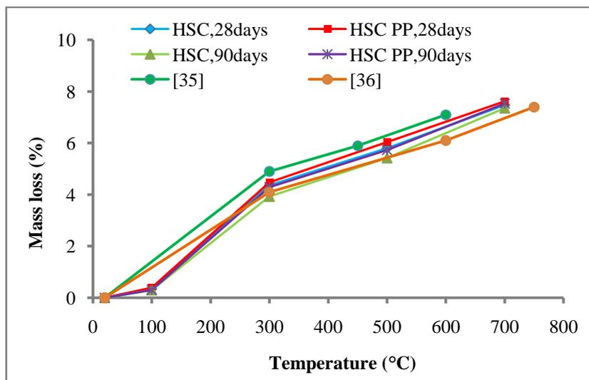
Figure.5. Mass loss as a function of temperature
