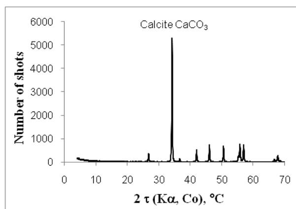
Figure.1. Diffractogram for limestone
