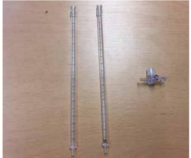
Figure 5. Manometer with three way tap (stopcock) used for the measurement of opening and closing pressures
