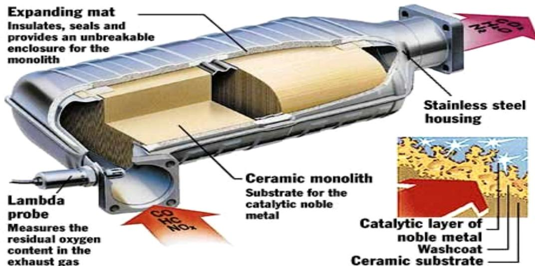
Figure 4: Structure of Catalytic converter.
