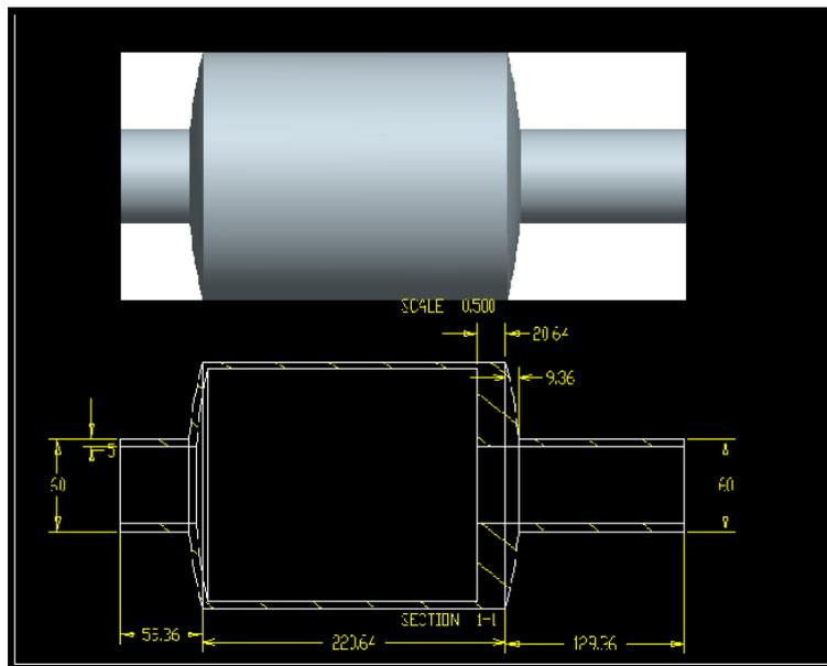
**Figure 2:** Outer design of converter.
